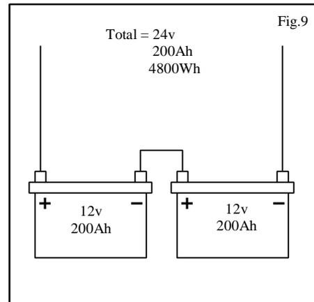
Leisure/Deep Cycle batteries are specifically designed for good performance in terms of charge/discharge cycles. Batteries are the most important part of your battery charging system and should be sized according to your load requirements and provide at least 3 days reserve capacity. This will reduce cycling, prolong the life of the battery and ensure system reliability during periods of low wind. *If in doubt about battery sizing, contact your dealer or the manufacturer.*
