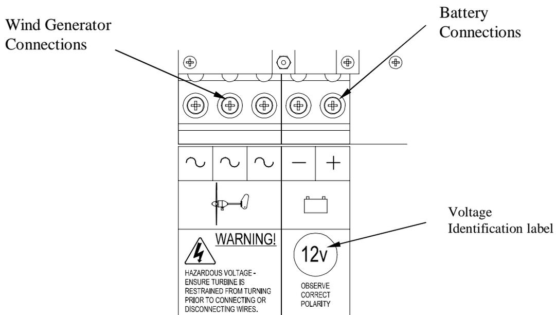
Fig 10. 12 & 24v Control Unit Connections
