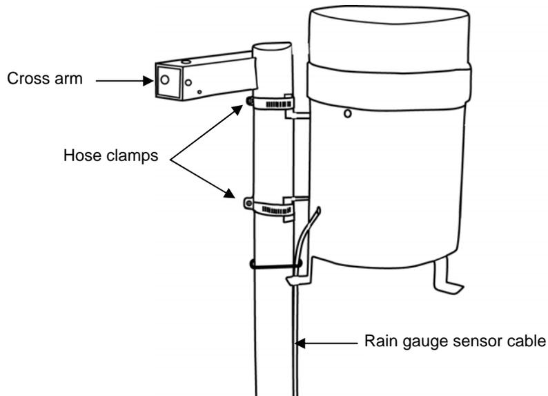
Figure 1: Rain Gauge sensor on the tripod mast
