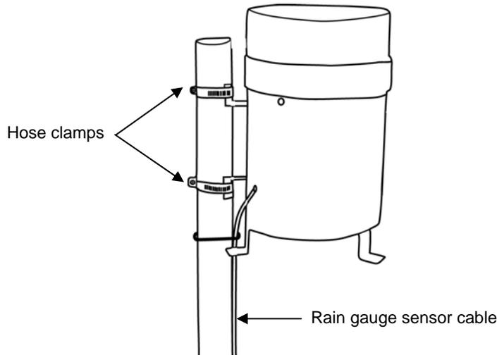
Figure 2: Rain Gauge sensor on separate mounting pole
