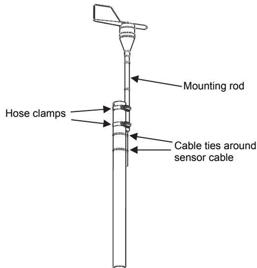
3. Tighten the hose clamps making sure the mounting rod remains vertical.
